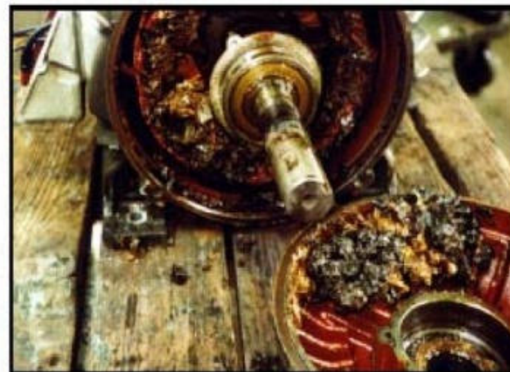
Figure 9. Over-greasing caused inside of motor to fill with grease.
